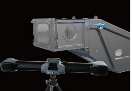
Its i-Tracker can be combined with tool simulators and path planning software to form M-Track, an intelligent robotic path planning and guiding system. The system comprises perception, planning, and execution modules, which cater to different applications such as grinding, coating, welding, and more.
