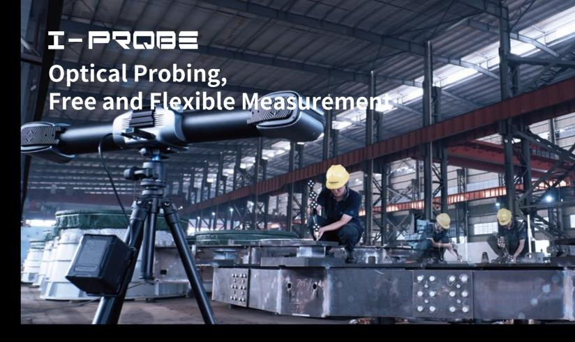
Tracking T-Probe comes with the i-Tracker to obtain dimensions of features, such as reference holes and hidden points. It can be widely used in the measurement of fixtures, stamping parts, and marking for actual machining allowance.
