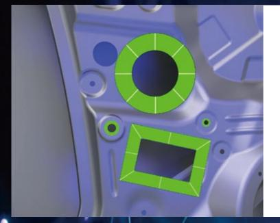
It boasts a shadow-less-light edge detection with high-precision gray value measurement. Users can inspect closed features precisely, especially threaded holes. Good measurements are ensured by delivering accurate and repeatable measurement results such as positions and diameters.
